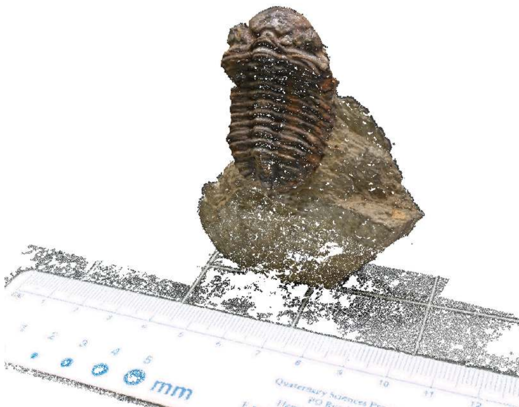
FIGURE 4. Dense point cloud of trilobite containing 179,294 points. Scale bar measuring millimetres is included in the point cloud.
