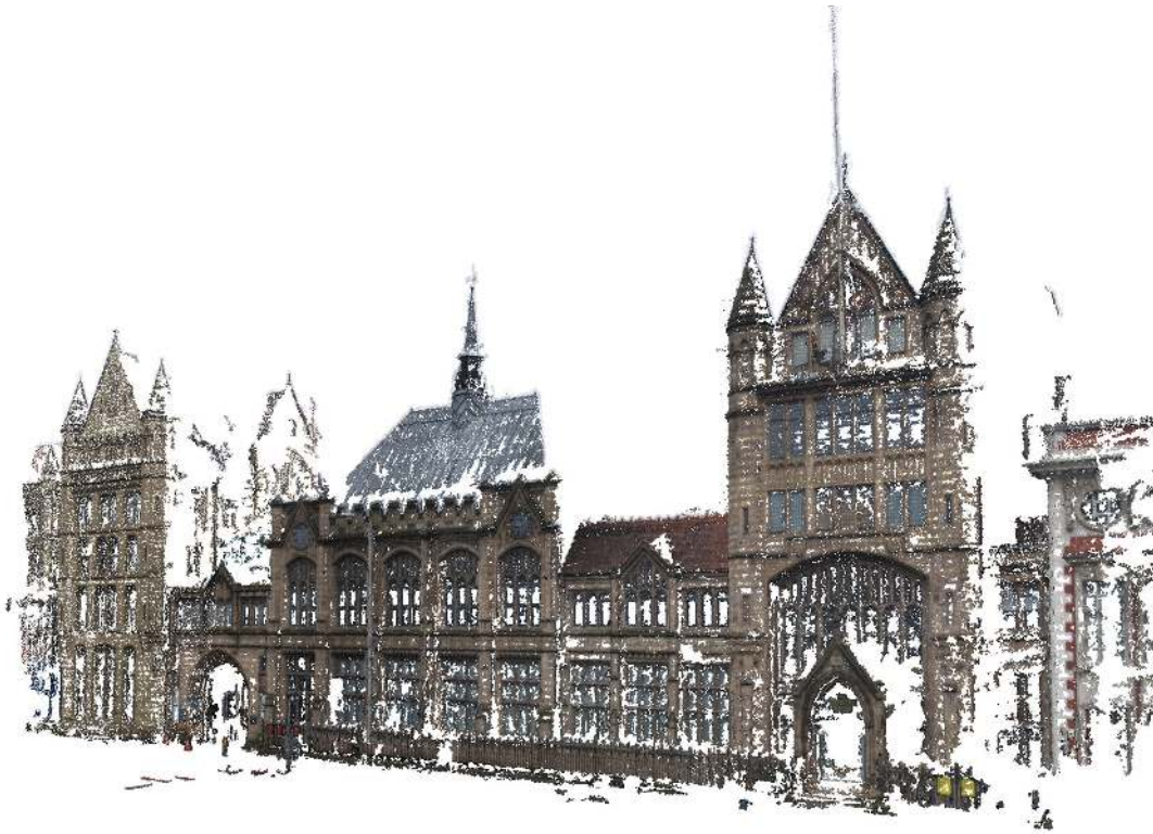
FIGURE 9. Dense point cloud of the Manchester Museum (Field of View ~ 60 m). This point cloud contains 1,070,573 points.
