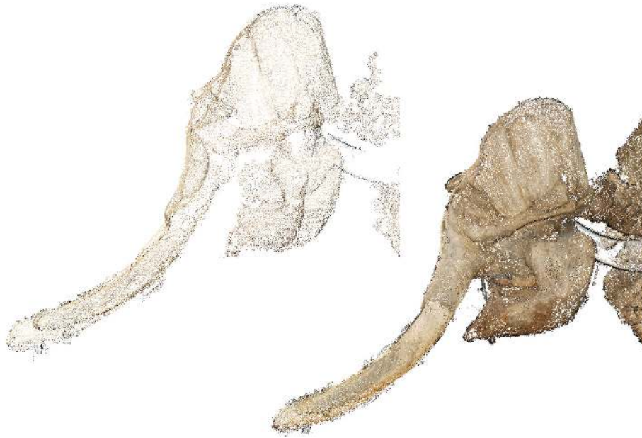
FIGURE 7. Comparison of dense point clouds produced using 44 (left) and 207 photographs (right). With additional photographs taken focusing on complex areas such as the jaw, the result is a considerably higher resolution point cloud.
