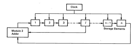
Pseudonoise digital modulation is used in a number of tracking and communications systems. In most cases it is necessary that the receivers of such systems bring an identical locally generated pseudonoise signal into time synchronism with the incoming pseudonoise signal. This acquisition process may require a relatively long time because of the period of the pseudonoise signals used and because of the autocorrelation properties of the signals.
