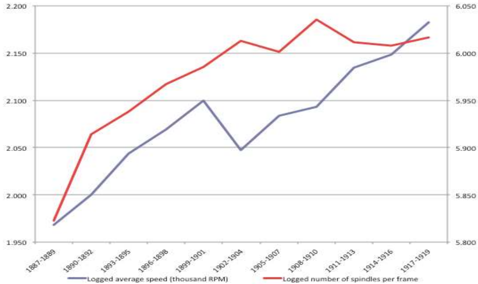
Figure A3. Dynamics of rotation speeds and spindles per frame on Japanese mills’ orders (log scale)
