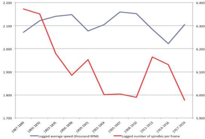
Figure A5. Dynamics of rotation speeds and spindles per frame on Indian mills' orders (log scale)
