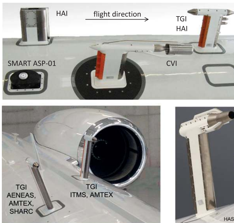
FIG. 3. Photos of parts of the upper fuselage of HALO. (top) Shown are the external structures of the hygrometer for atmospheric investigations (HAI), the trace gas inlet (TGI), and the HALO counterflow virtual inlet (CVI). The upward-looking irradiance optical inlet of the spectral modular airborne radiation measurement system (SMART) is also depicted. (bottom left, bottom right) The two TGIs and the HALO aerosol submicrometer inlet (HASI) are pictured.
