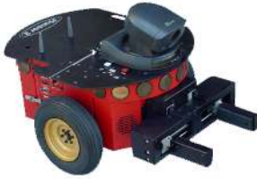
Figure 5: A typical prototype of Pioneer 2-DX robot with gripper
