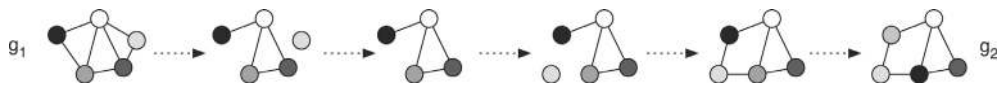
Figure 2.1: An example edit path between g_1 and g_2 (node labels are represented by different shades of gray). Image courtesy of Kaspar Riesen [111].
