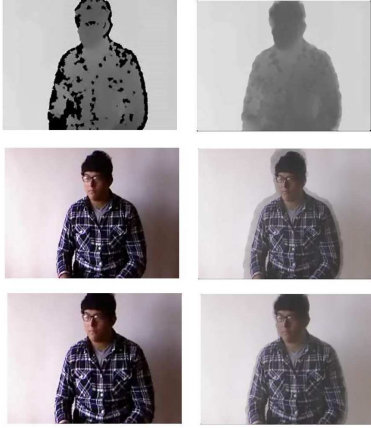
Figure 1: 1st row: inpainting+HMF results of a depth sample from isoGD [35] dataset. 2nd row: superposition before registration. 3rd row: superposition after registration.
