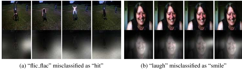
Figure 5: Incorrectly classified video frames showing attention over time: The white regions are where the model is looking and the brightness indicates the strength of focus.
