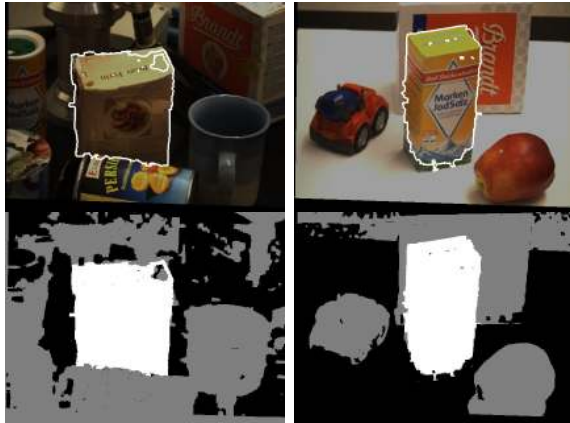
Fig. 6. Segmentation results without an obvious surface plane. The lower images show pixels labeled as surface points in gray.
