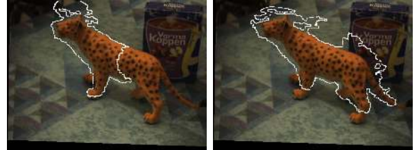
Fig. 9. Segmentation results without color measurements. The images show the 1st and 7th frames of a sequence.
