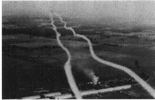
Figure 5.4 Instability of trailing vortices visualized by smoke [5.4]. View from chase airplane.
