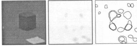
Fig. 4. Zooming in to a region of interest obtained from a dark blob extracted by the scale-space primal sketch. (a) A window around the region of interest, set from the location and the size of the blob. (b) The rescaled level curve curvature computed at the scale given by the scale-space blob (inverted). (c) The boundaries of the 20 most significant curvature blobs obtained by extracting dark blobs from the previous curvature data.
