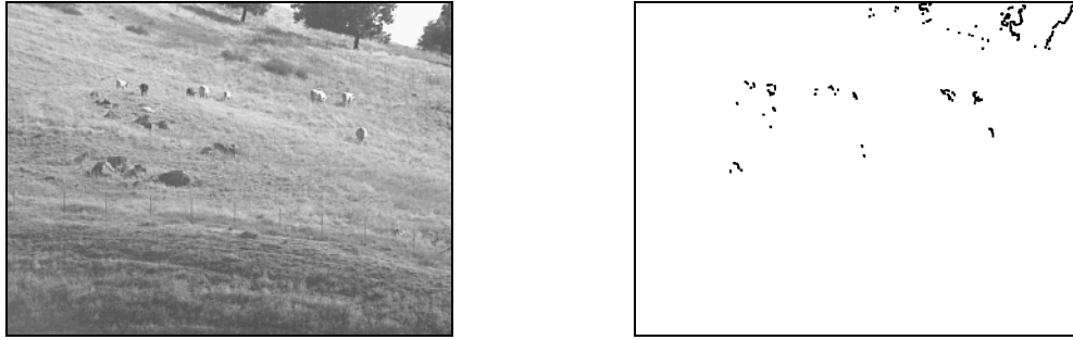
Figure 4-3 Edge detection in a scene outside the IBM Almaden Research Center. On the left is the raw image and on the right are the edges detected with a brightness threshold of 75. The data is a set of snapshots from IBM Almaden's CattleCam [Almaden97] and the application attempts to detect cows in the landscape above San Jose.
