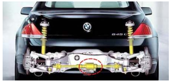
Figure 2. Illustration of the active roll control (ARC) system of BMW using a hydraulic rotary actuator [14]
