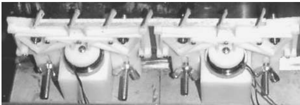
Fig. 8 High-frequency, deployable MVG test hardware.
