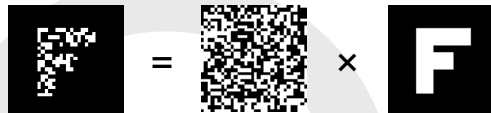
Fig. 7. Example of one of the projected images, representing the product between a random measurement pattern and the image to be reconstructed.
