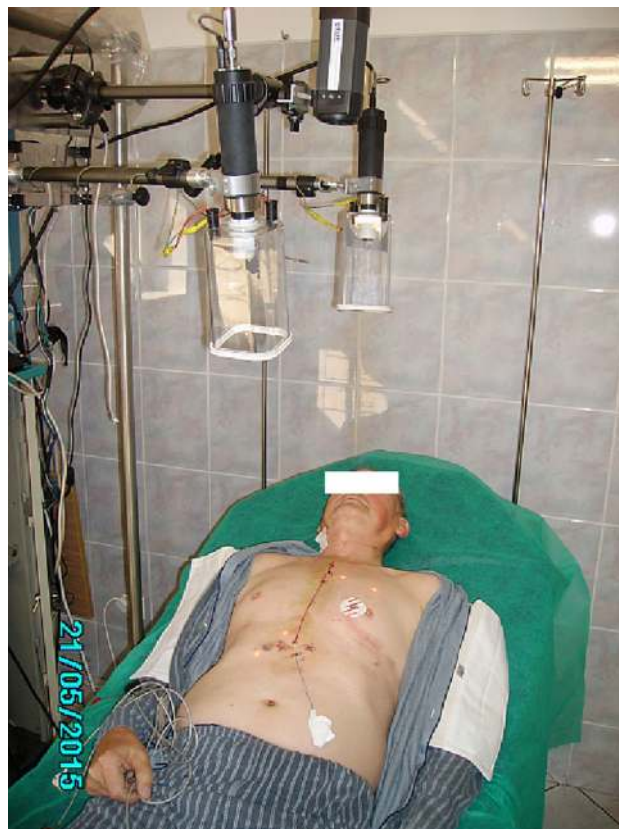
Fig. 4 The experimental ADT set-up in clinical environment, visible are cooling heads and IR-camera (LW FPA, uncooled)
