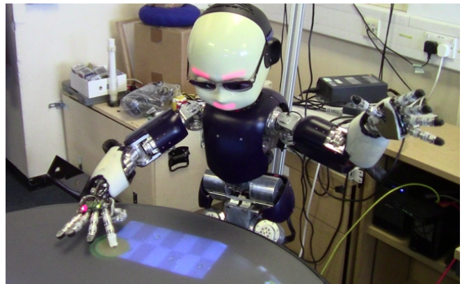
Fig. 1. iCub interacting with the virtual keyboard shown by the Reactable tactile interface. The finger is used to control the virtual object, which is used by our software to know which sound to play.
