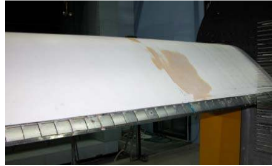
Fig. 3-9 Wind-tunnel model with trailing edge ATEG. (Photo by Risoe DTU National Laboratory for Sustainable Energy 39 )
