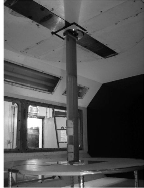
Fig. 3-11 DUWIND's "smart blade" experiment tested at TU Delft LSLT wind tunnel. (Source: Barlas and van Kuik 4 )
