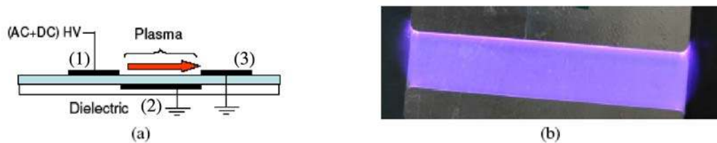
Fig. 3-32 a) Schematic side view of three-electrode discharge actuator, b) top view of produced discharge. (Source: Moreau et al. 93 )
