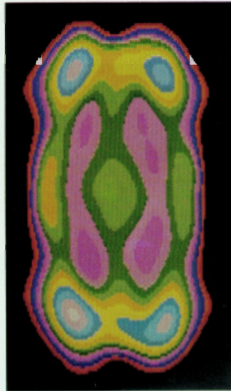
Fig. 8. Section of simulated human arm (upper segment) surrounded by water. Reconstruction (modulus of \tilde{K}(x, y) ).
