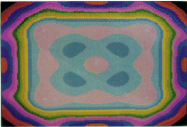
Fig. 7. Square object composed with fat, muscle, and bone surrounded by water. Reconstruction (modulus of \tilde{K}(x, y) ) displayed on a TV monitor.
