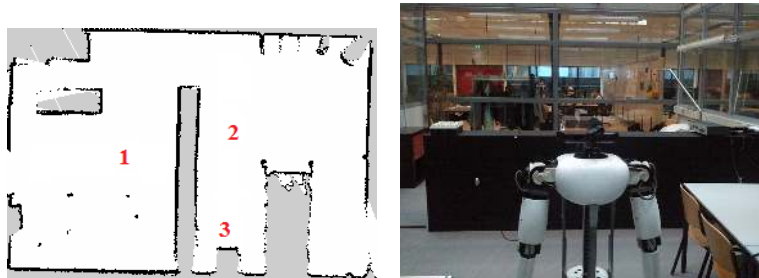
(a) Occupancy grid map of the lab in which the search takes place. (b) Photograph of the lab with AMIGO from the entrance.
