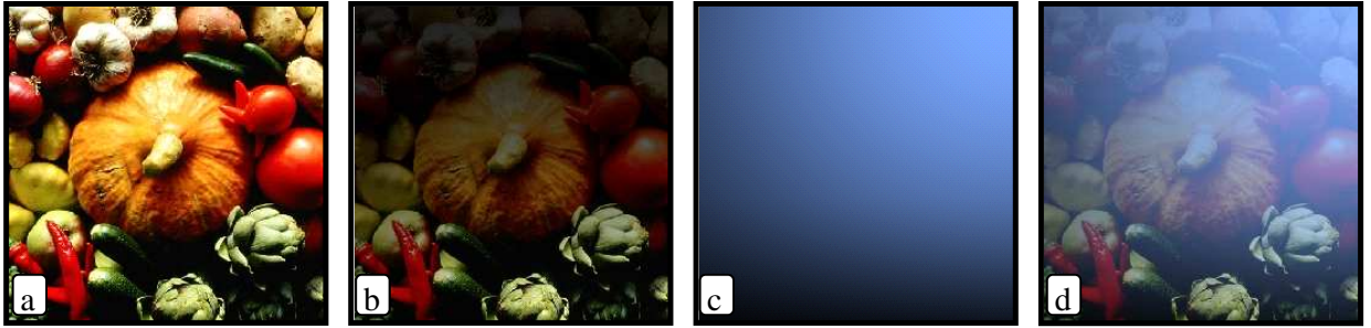
Fig. 2. Simulation of an underwater scene. The scene was assigned a linearly varying distance map ranging between [0.2m, 1m] . (a) A uniformly lit clear scene. (b) The simulated attenuated signal. (c) The backscatter component. (d) The sensed underwater scene, accounting for both scattering and attenuation.
