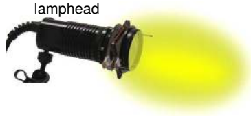
Fig. 3. An example of an anisotropic illumination pattern Q(\mathbf{X}) : Even in the same radial distance from the lamphead, the lighting changes laterally.
