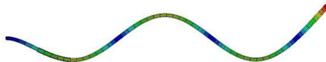
Figure 13 Mode shape of beam (c) using 2D-FE (ABAQUS)
