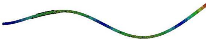
Figure 12 Mode shape of beam (b) using 2D-FE (ABAQUS)
