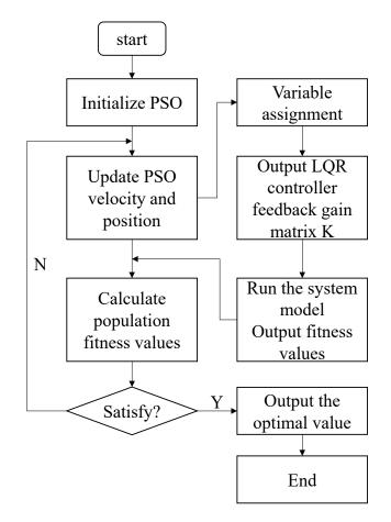
Figure 4. Flow chart of the PSO algorithm optimize LQR parameters.
