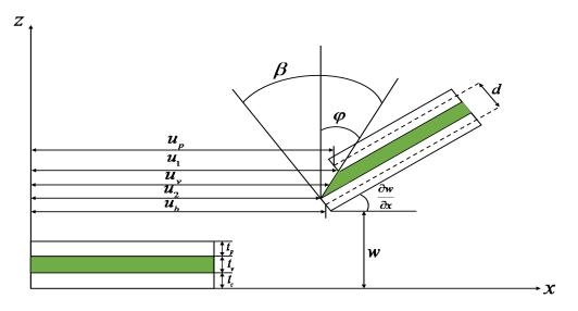
Figure 2. Geometric deformation relation of ACLD cantilever beam structure.
