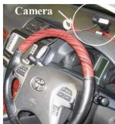
FIGURE 2. Webcam on vehicle fascia for capturing facial cues.
