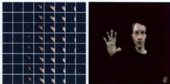
Fig. 6. The skin tone filter responds to 4.7% of possible (R, G, B) values. Each grid in the figure to the left shows the response of the filter to all values of red and green for a fixed value of blue. The image to the right shows the filter in operation. Typical indoor objects that may also be consistent with skin tone include wooden doors, cream walls, etc.
