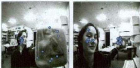
Fig. 8. Effect of gain adjustment on looking preference. Circles correspond to fixation points, sampled at one second intervals. On the left, the gain of the skin tone filter is higher. The robot spends more time looking at the face in the scene (86% face, 14% block). This bias occurs despite the fact that the face is dwarfed by the block in the visual scene. On the right, the gain of the color saliency filter is higher. The robot now spends more time looking at the brightly colored block (28% face, 72% block).
