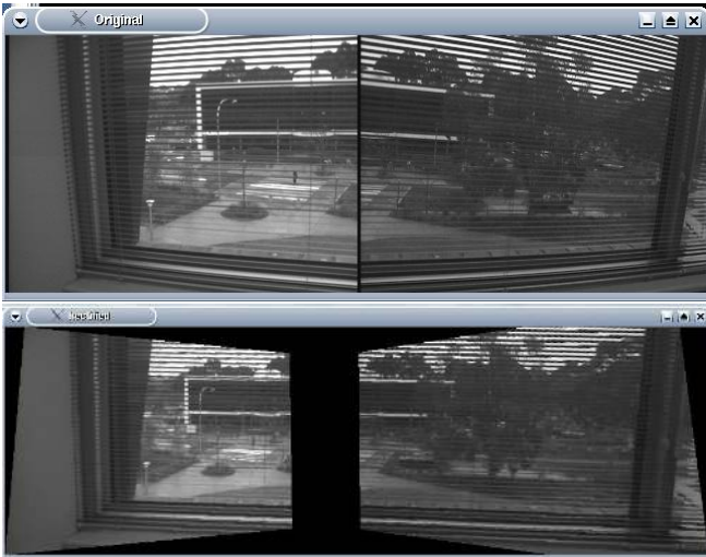
Figure 5: A scene viewed through blinds showing the output of the active rectification process. Top: original left and right images. Bottom: images warped such that parallel epipolar geometry is enforced.
