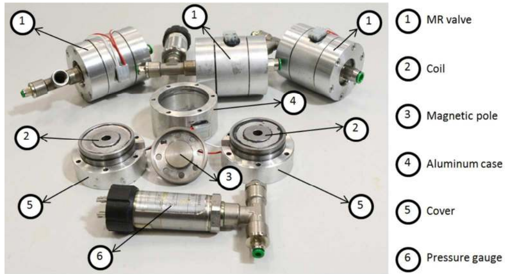
MR valves picture with description of parts [insert figure 13] 147x80mm (300 x 300 DPI)
