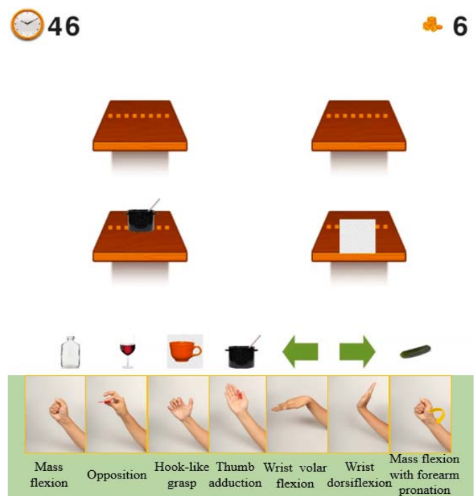
Fig. 2. A serious game “ Get objects from the shelf ” for ADLs-based upper limb motor function rehabilitation. Seven different objects can appear on eight different positions on the shelf which is in front of the user. The object on the shelf is regarded as the target of the current round, and the user reaches for the correct position and then performs mass flexion, opposition, hook-like grasp, thumb adduction, wrist volar flexion, wrist dorsiflexion, or mass flexion with forearm pronation to complete the correct movement in the game: grasp a bottle, hold a glass of wine, grab a cup with handle, grab a spoon, turn left, turn right, or grasp a cucumber with forearm pronation, respectively. The gray pictures indicate the current estimated position and target object, which allows the user to adjust his movement to complete the target successfully.
