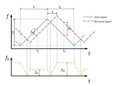
**Figure 2.** The curve of the beat frequency versus time.
