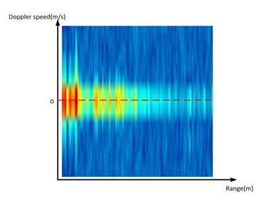
Figure 3. The visualization of range–Doppler data.
