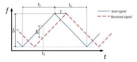
Figure 1. The curves of the sent signal frequency and the received signal frequency versus time.
