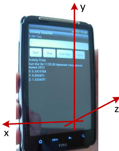
Figure 7: Smartphone is in vertical position. Acceleration along y-axis. x: 0.6403563, y: 9.806434 \approx 1g, z: 1.6334297
