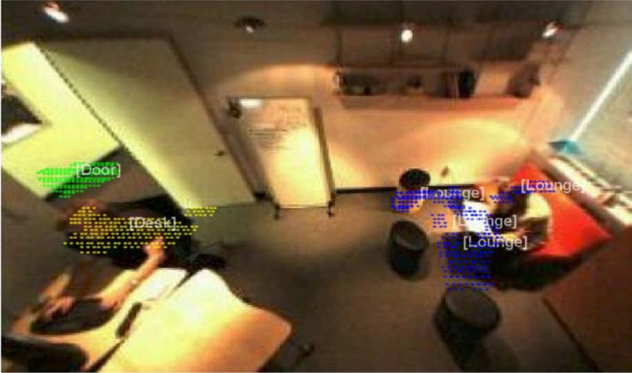
Fig. 10. The workspace overlaid with clustered tracker data for three different zones; zone labels (door, desk, lounge) are user-supplied
