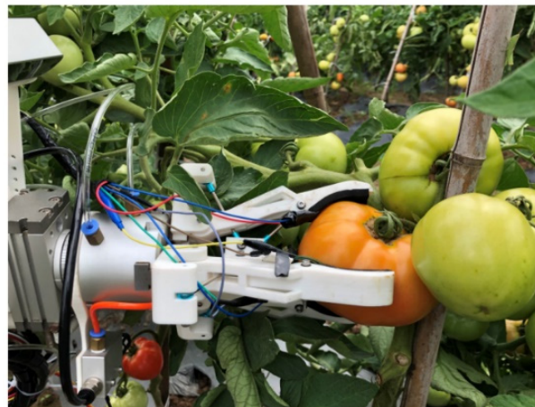
Figure 5. Tomato picking end-effector based on non-destructive pneumatic clamping control [67].
