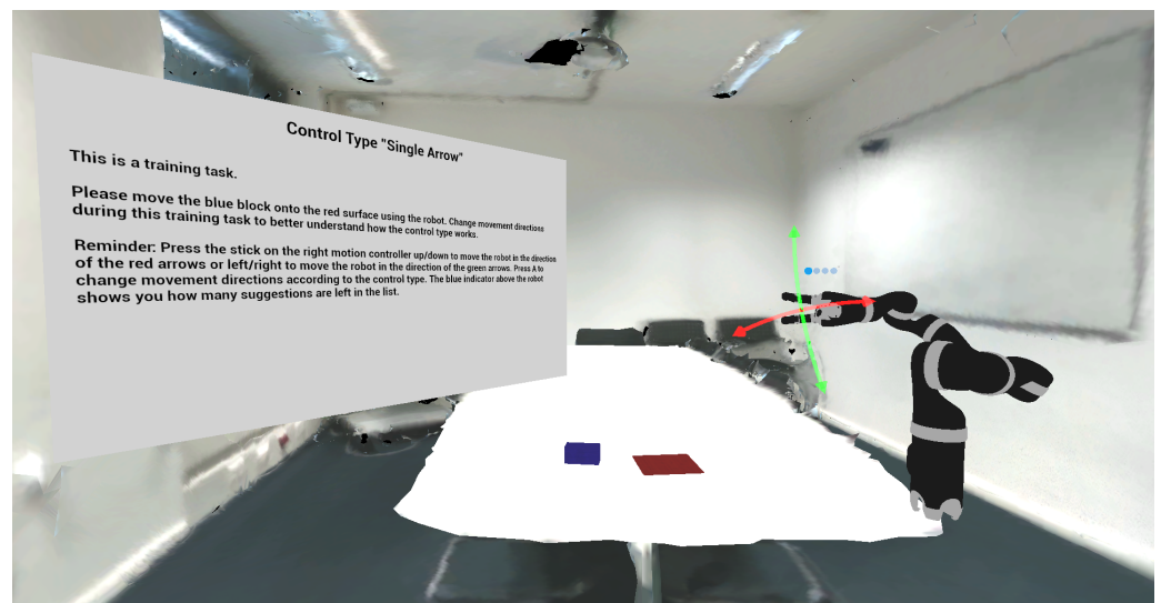
Figure 5. The virtual environment: description screen ( Left ); screen with example photos of the control types (not shown); Kinova Jaco with visualisation for control type Single Arrow ( Right ); table with blue block and red target ( Bottom ).
