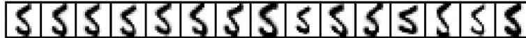
Fig. 1. Example of first-order approximation of affine transformations and line thickness. (Left to right: original image, \pm horizontal translation, \pm vertical translation, \pm rotation, \pm scale, \pm diagonal deformation, \pm axis deformation, and \pm line thickness).
