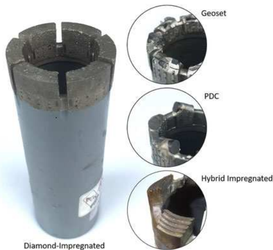
Fig. 4. Winkie Drill is equipped with four bit designs. The #10 diamond-impregnated bit is used in hard bedrock formations. The geoset bit is used in soft rock formations or when sediments are entrained in the ice. The PDC bit can be used in similarly soft rock formations but has had limited success when ice is present in the kerf. The hybrid impregnated bit is made from the same material as the standard #10 diamond-impregnated bit but includes a relief angle behind the leading edge. This bit can cut ice and transition into bedrock.
