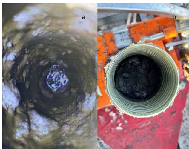
Fig. 9. (a) Warm fluid near the bit resulted in an eroded borehole wall. (b) The water refroze further up in the casing, resulting in flakes that plugged the casing.
