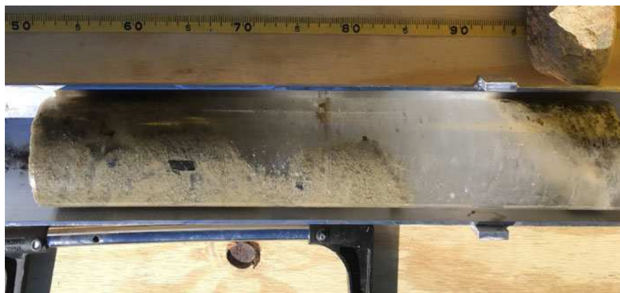
Fig. 8. Core at Ong Valley was especially complicated to drill because it very quickly changed from clean ice, to thin clay layers, to rocks several centimeters in diameter.
