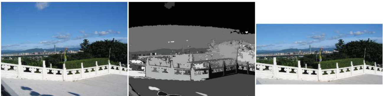
Fig. 3. Automatic cropping of irrelevant borders: original image (left), detected regions (middle), cropped image (right).
