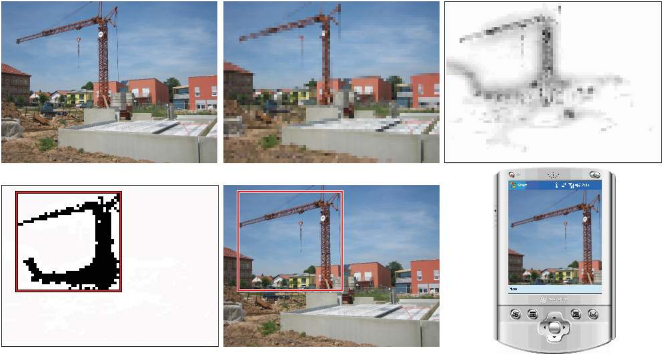
Fig. 5. Automatic detection of relevant regions based on saliency maps.
