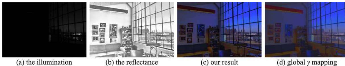
Fig. 7 Validation of the proposed tone mapping algorithm: (a) Illumination estimation, in which the abrupt variations of the original intensity are mainly encoded. (b) Corresponding reflectance map in linear space, which has a much lower dynamic range than the original map and the illumination estimation. (c) Tone-mapped result produced by the proposed algorithm, where fine details can be perceived without visible artifacts. (d) Globally mapped image using the same \gamma as in producing (c). However, details are diminished.
