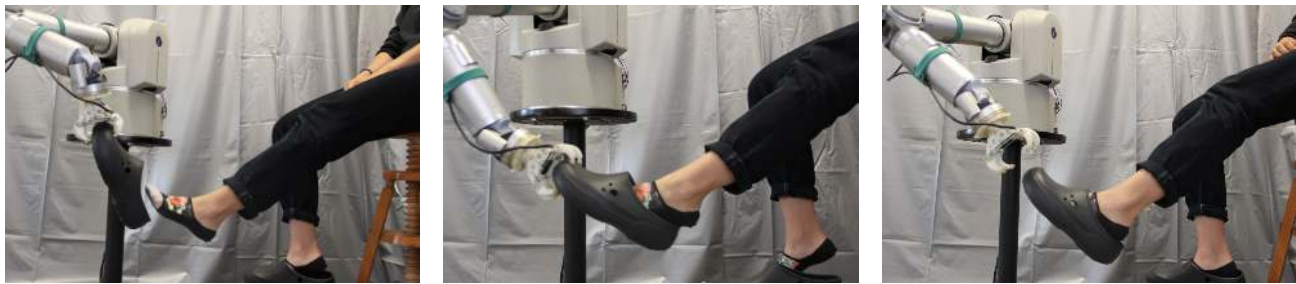
(a) Approach action, to get closer to the foot. (b) Insert shoe action, using an elaborated wrist rotation (see supplementary video). (c) Release action, to move away.
