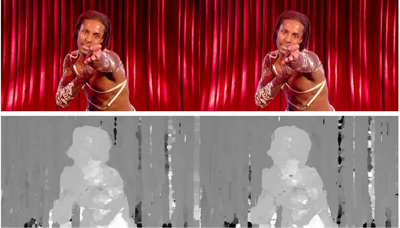
Figure 5. Top row: the left and right rectified images from the original stereo pair (pictures courtesy of Binocle). Bottom row: the left and right disparity maps produced from these images by a basic method, obviously containing many matching errors.
