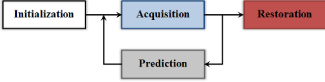
Fig. 2. Scheme of an adaptive acquisition framework for single-pixel camera.
