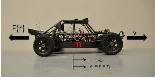
Fig. 3: Dynamics on a free body diagram of a vehicle
