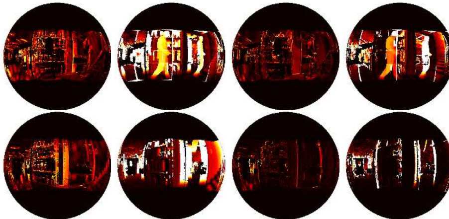
Fig. 6: Intensity and geometry errors between indoor frames with a gap of fifteen frames for two different scenes. Each row is composed of two pairs of errors: the classic RGB-D and the adaptive formulation in the form (\mathbf{e_I}(\mathbf{x}), \mathbf{e_D}(\mathbf{x})) .
