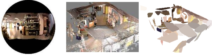
Fig. 3: Spherical intensity image (left), point cloud (middle) and segmented patches (right) of rendered indoor scene using the superpixels constraints. For display purposes, plane colors are the average color of each patch. The segmentation preserves edges as the calibration target and whilst reducing the noise in frontier stitched regions.
