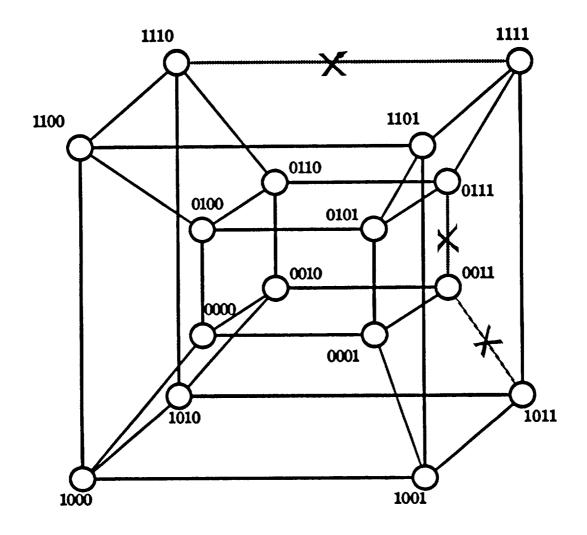
Figure 5 . An injured  $Q_4$  where links 0-11, -011 and 111- are faulty.
