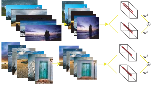
Figure 5: Grouping strategy to reduce computational overhead: The integer dilated Convs can be shared by properly grouped images according to aspect ratios.
