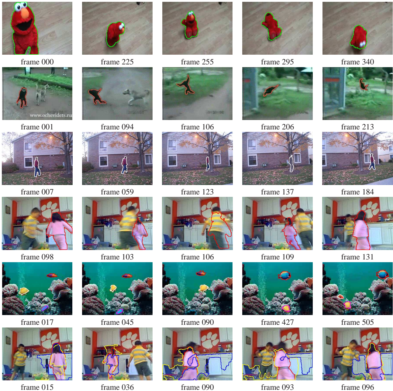
Figure 5. The top two rows shows the results of our algorithm on the Elmo and Monkey sequences, in which target undergoes shape deformation and large unpredictable motion. The next two rows shows results on sequences in which a person walks behind a tree and a girl runs in circles around a room; the hallucinated contour is shown when the target is completely occluded, in frames 137 and 106, respectively. The fifth row shows the results of a sequence in which multiple fish swim in a tank and are all tracked successfully by the algorithm. Note especially the camouflaged small blue fish (magenta outline) at the bottom of frames 017 and 045. The last row shows the comparison of our results (red contour) with Linear RGB Histogram [6] (yellow) and standard color histogram [21, 22, 13, 19] (blue) on the girl sequence.
