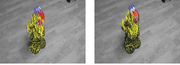
Figure 4. Joint Lucas-Kanade (right) produces smoother motion vectors than standard Lucas-Kanade (left). The vectors are colored by the fragment in which they are contained.
