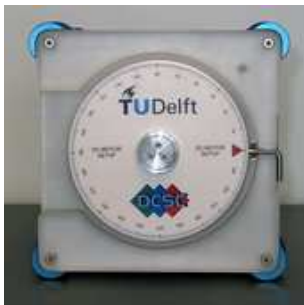
Fig. 5: Servo positioning system with a manually adjustable level of friction (using the lever at the right side of the box).
