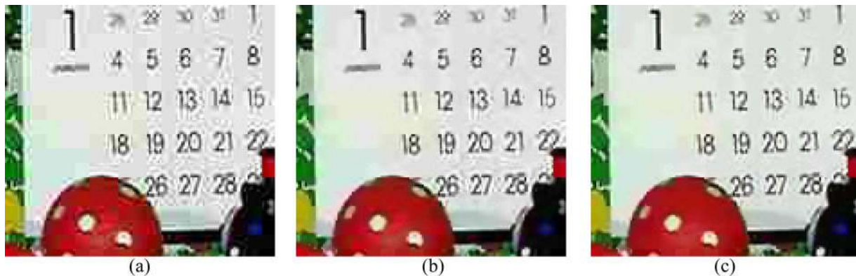
Fig. 16. Zoomed views for images in Fig. 15. (a) Compressed; (b) fuzzy spatial filter; (c) proposed fuzzy spatiotemporal filter.
