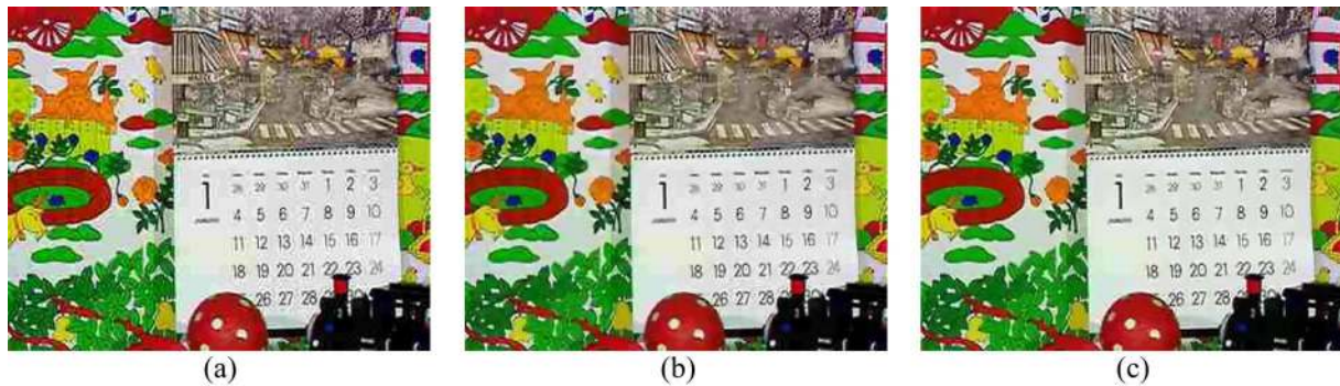
Fig. 15. Comparison of filter results for MJPEG sequences. (a) Compressed (21.22 dB); (b) fuzzy spatial filter (21.50 dB); (c) proposed fuzzy spatiotemporal filter (21.89 dB).
