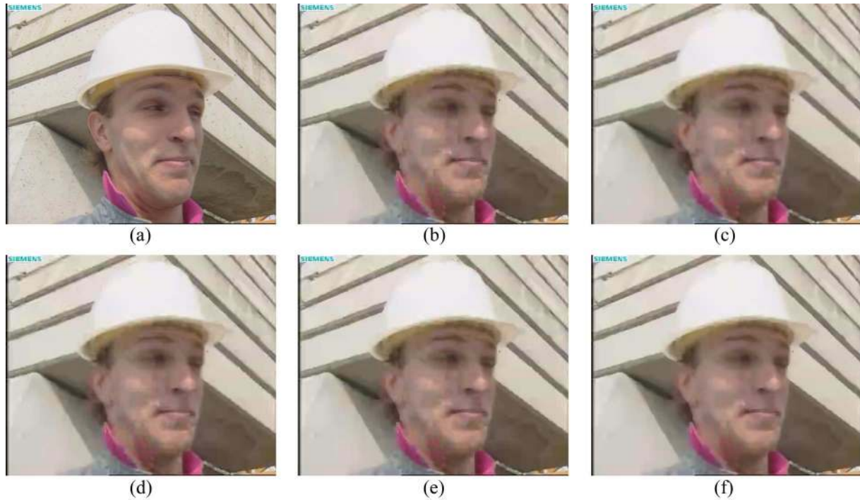
Fig. 19. Comparison of filter results for H.264 sequences. (a) Original frame; (b) compressed (30.77 dB); (c) Chen's method (30.37 dB); (d) Liu's (30.51 dB); (e) fuzzy spatial filter (30.90 dB); (f) adaptive fuzzy MCSTF (31.09 dB).
