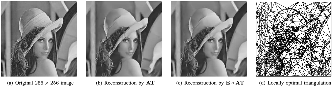
Fig. 2. Test image Lena. Comparison between compression methods AT and E o AT , whose image reconstruction is shown in (b) for AT at 0.279 bpp with PSNR 28.77 dB and in (c) for E o AT with PSNR 29.19 dB. The locally optimal Delaunay triangulation output by E o AT is shown in (d).
