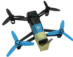
Fig. 6 The container attached to the nose of the quadrotor with one weight inside.
