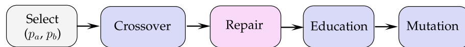
Fig. 4 Generation of a child solution in AMA-VRPTW. The repair procedure is executed only if the child is not feasible (rendered in light pink) (color figure online)
